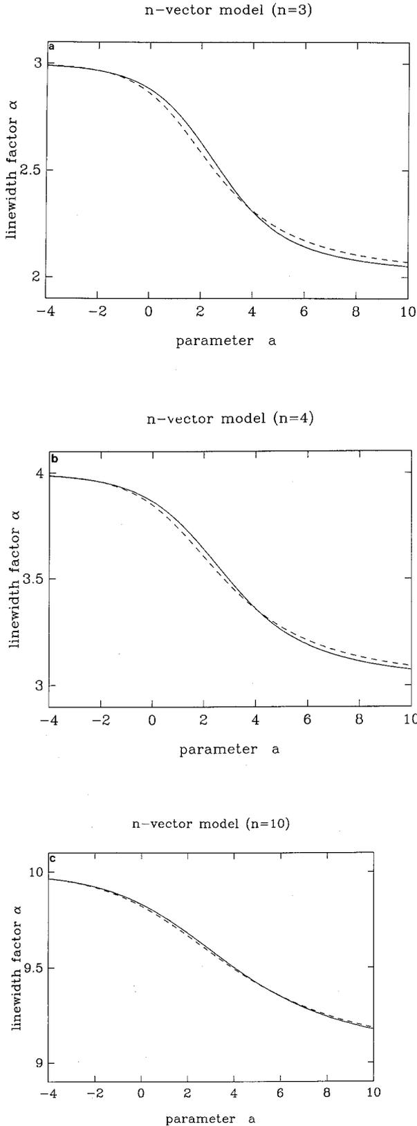
**Fig. 1a-c.** Linewidth factor  $\alpha$  vs. control parameter  $a$  for (top)  $n=3$ , (middle)  $n=4$ , and (bottom)  $n=10$ ; (solid line) is our result from a numerical solution of (19) and (20); (dashed) is the result of Ziegler and Horner's analytical approximation [12], (8)
